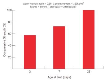
Note data is based on concrete mixes containing no admixtures or other cement extenders e.g. flyash, blast furnace slag. Use of such products will alter the strength development characteristics of concrete containing GP Cement.
